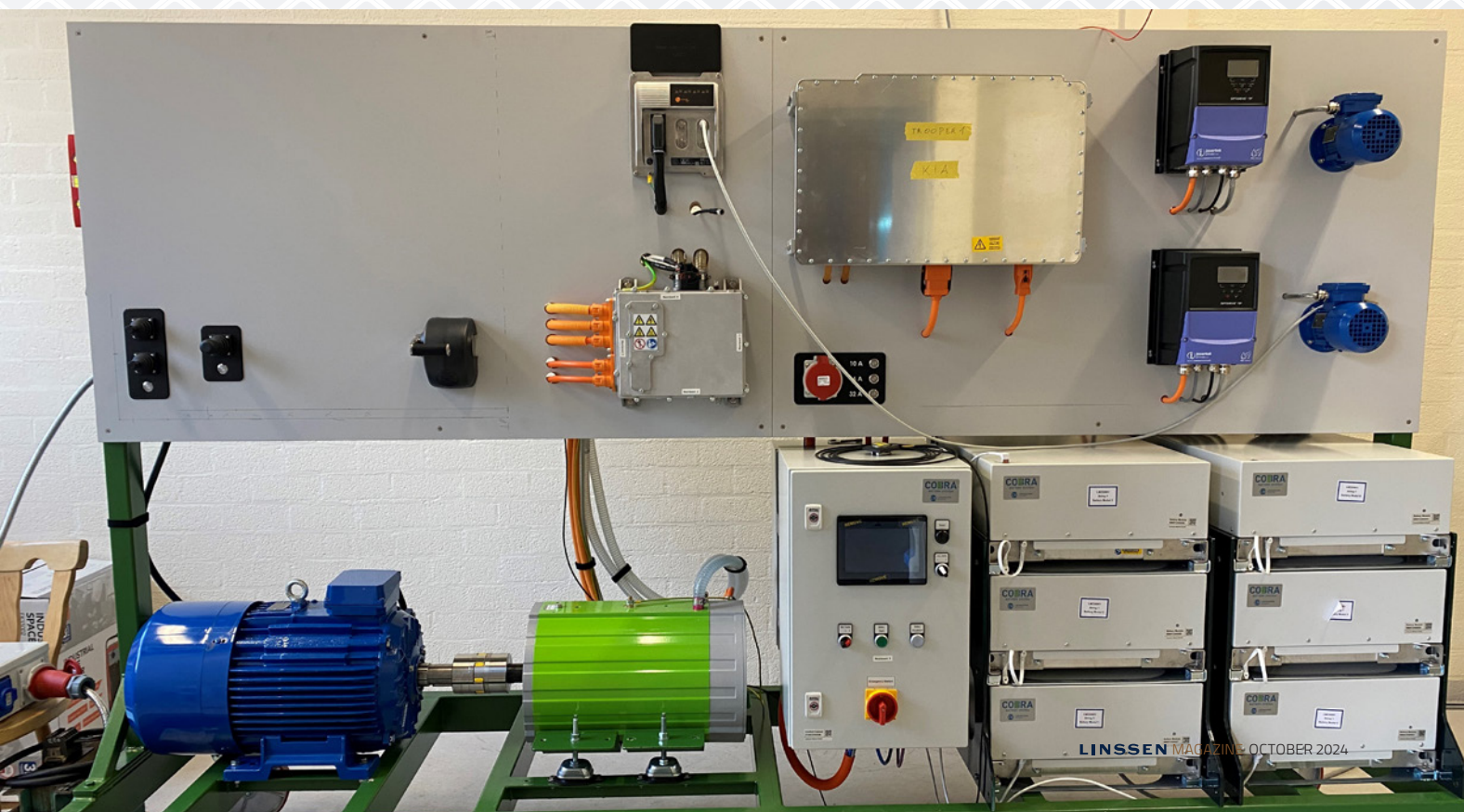
Test set-up of the different modules in the development of the Linssen electric drive.
