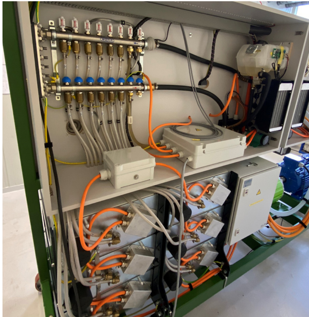
Test set-up of the different modules in the development of the Linssen electric drive.
